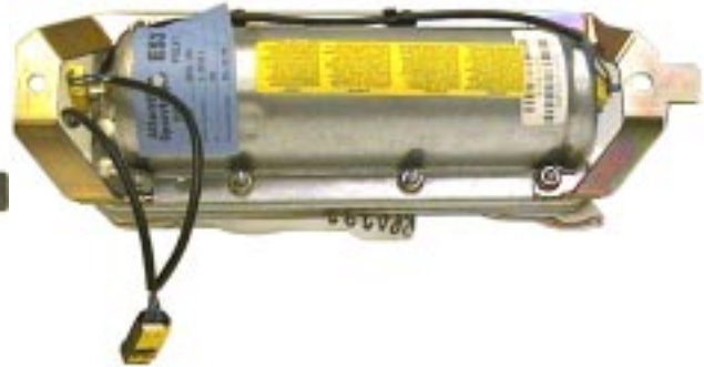
2-Stage Passenger Airbag (Rear View)
